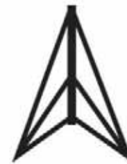
(c) Cable bracing
